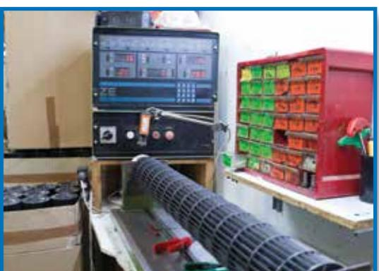
Ultrasonic welding machines for plastic fans production and fan balancing machines for precise parts production.
