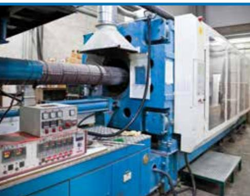
CNC Automated Injection machines production line for plastic parts, capable of producing parts weighting from 10 gr up to 6.5 kgr.
