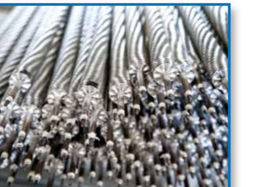
Electrical heaters production line for Air curtains.
