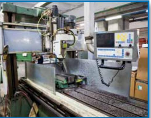
PRO Engineer Software station for MOULD design connected with a 4 AXIS CNC mill with a long up to 3 meters table for big Moulds production.
